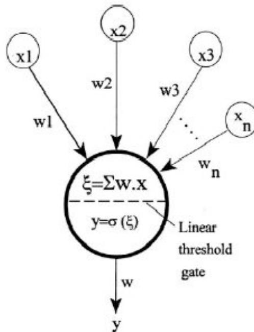
Figure 2. A schematic of the “Perceptron”, a common node in artificial neural networks. (From [2])
