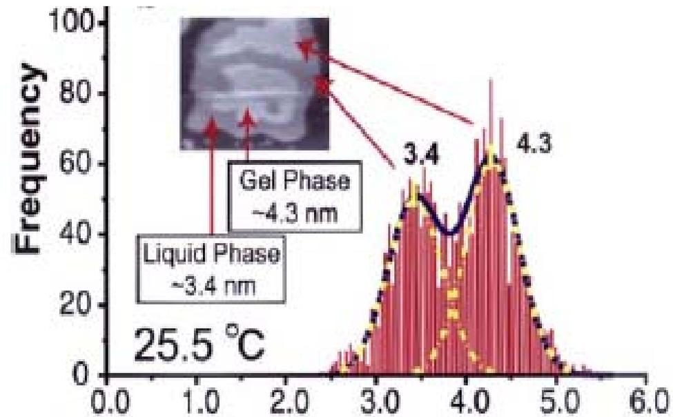
AFM-derived height profiles during a temperature-induced phase transition of a DMPC membrane can be represented as Gaussian distributions. A  $1.4 \times 1.4 \mu\text{m}$  area was analysed from three consecutive  $10 \times 10 \mu\text{m}$  images collected at a heating rate of  $0.11^\circ\text{C}$ .
