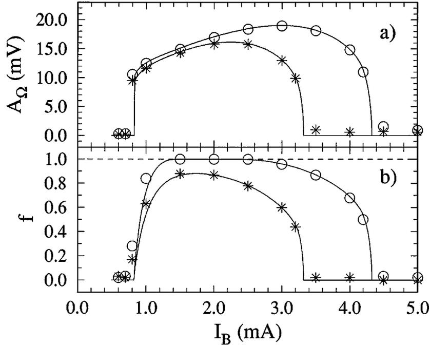
Fig. 6) Dependence of  $A_\Omega$  (a) and  $f$  (b) on  $I_B$  at  $\Delta = 0.001$ mA (circle) and  $\Delta = 0.002$ mA (asterisks) based on Kirchoff Eqns (13). Solid line represents analytic Eqn (17) and (19) [1]
