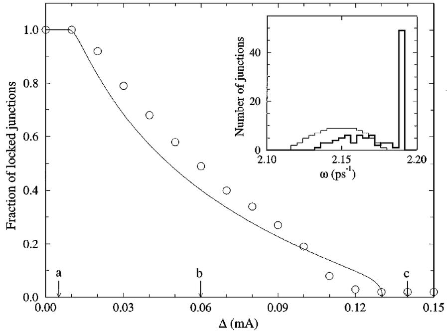
Fig. 6) Fraction of phase locked junctions with typical parameters for Josephson junctions. Circles are from the numerical calculations and solid line is analytic result, Eqn (17). Inset: bare frequency (thin) and dressed frequency (thick) distributions at (b)  $\Delta = 0.06$  [1].
