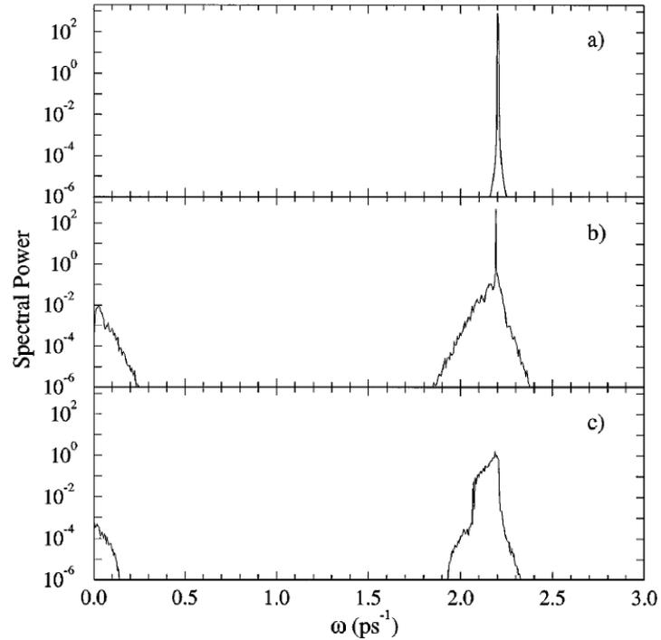
Fig. 7) Power spectra for the whole array at different values of  $\Delta$ , given by  $(\hbar/2e)(\sum \dot{\phi}_k - \langle \sum \dot{\phi}_k \rangle)$ . A peak around  $\omega \approx 2.2$  grows as the system goes from (c) to (a) phase in Fig. 6 [1].
