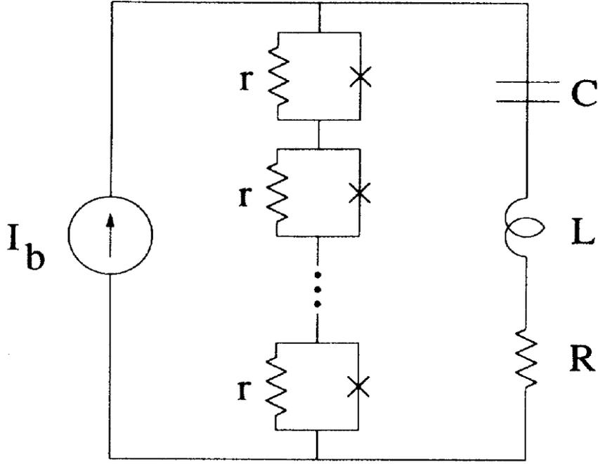
Fig. 5) Circuit schematic of series array of Josephson junctions [9]
