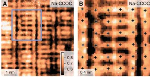
Figure 7: Charge order seen in under-doped cuprates [9].
