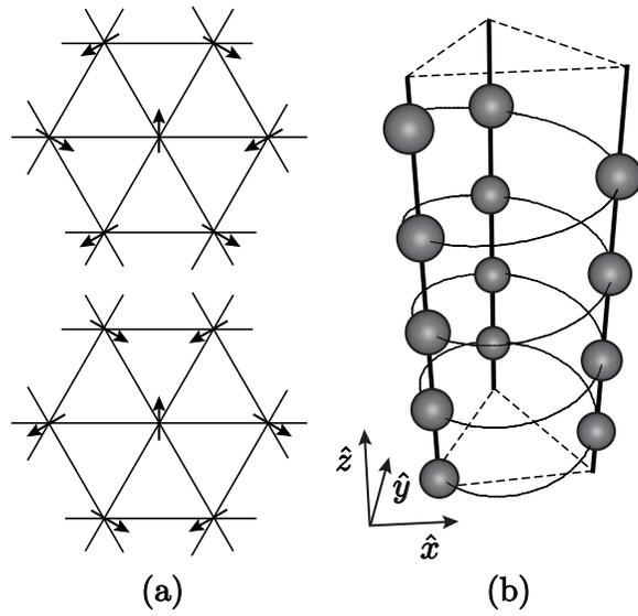
Figure 3: Correspondence between polyelectrolyte bundle and  $T = 0$  2D JJ array. (A) The two degenerate, chiral ground states of the antiferromagnetic XY model on a triangular lattice. The helical ordering around a triangular plaquette of the bundle lattice is shown in (B), where the dark black lines depict the polymer backbone while the spheres depict peaks in the condensed charge density [9].
