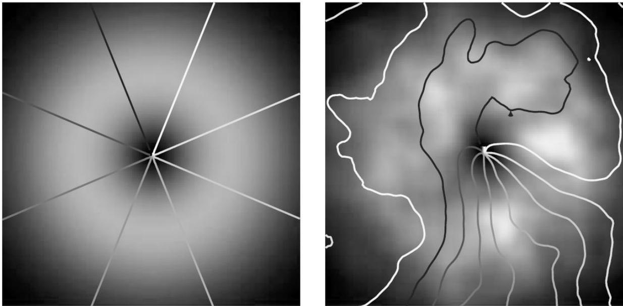
**Figure 4:** Images showing lines of constant phase on a beam with topological charge of 1. The image on the left shows the initial beam, without propagating through any atmospheric turbulence. The right image shows the effect of the phase aberrations on the beam. Figures from Ref. [6].
