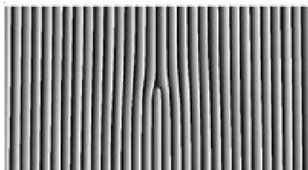
**Figure 3:** Image of a computer generated hologram that shows. Diffraction off of this hologram changes the angular momentum state of a photon. By doing so, the angular momentum state can be detected. Figure from Ref. [4].
