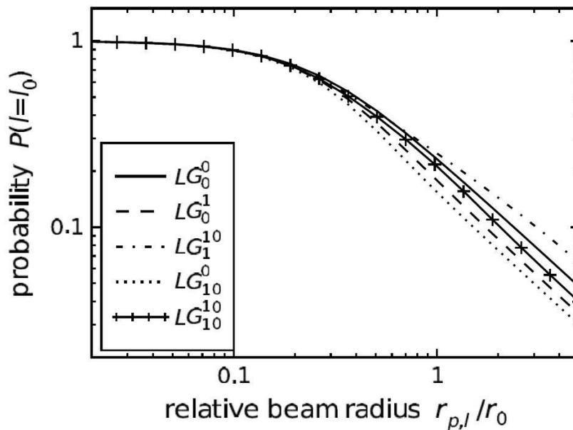
**Figure 6:** A plot summarizing the relevant analysis by Paterson. Here, the convention is  $LG_{|m|}^p$ , where  $m$  refers to the topological charge, and  $p$  is the radial mode. The x-axis is the ratio between the rms beam radius and the Fried parameter (the length scale that turbulence becomes important). Figure from Ref. [6].
