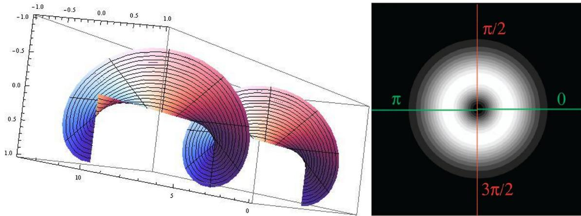
**Figure 2: a)** An image of the wavefront of a photon with a topological charge of 1. A larger charge would cause the rotation to be faster, whereas a negative charge would cause the rotation to be in the reverse direction.
