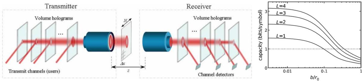
**Figure 1: a)** A diagram showing the multiplexing of multiple systems using angular momentum states and holograms to combine or pick off the specific angular momentum component. Depending on the stability of the other source of bits, either the angular momentum can be used to combine multiple channels or as additional bits. Figure from Ref. [5].
