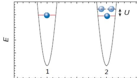
**Figure 1:** If the atom in site 1 hops to site 2, there will be an energy cost of  $U$  due to the repulsive interaction between two atoms in site 2 [3].
