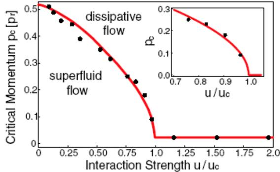
**Figure 11:** Critical momentum for a condensate in a 3D lattice. The solid line shows the theoretical prediction for the superfluid region. The horizontal solid line is a fit to the data points in the mott-insulating phase. (Inset) Fit of critical momentum near the superfluid to mott-insulating transition [6].
