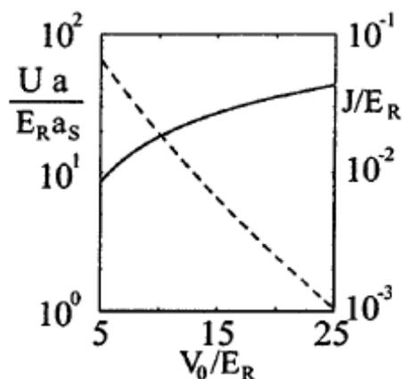
**Figure 2:** Plot of the scaled on site interaction  $U/E_R$  multiplied by  $a/a_s$  ( $\gg 1$ ) (Solid line; axis on left-hand side of graph) and  $J/E_R$  (dashed line; axis on right-hand side of graph) as a function of  $V_0/E_R$  [1].
