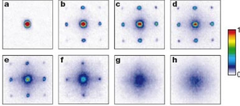
**Figure 6:** Absorption images of multiple matter wave interference patterns. These were obtained after suddenly releasing the atoms from an optical lattice potential with different potential depths  $V_0$  after a time of flight 15ms. Values of  $V_0$  were: a,  $0E_R$ ; b,  $3E_R$ ; c,  $7E_R$ ; d,  $10E_R$ ; e,  $13E_R$ ; f,  $14E_R$ ; g,  $16E_R$ ; h,  $20E_R$ ; [3]
