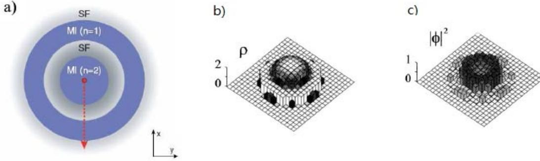
**Figure 4:** a) wedding cake structure of superfluid and mott-insulating phases; b) the density of cold atoms; c) the superfluid component. Parameters:  $U = 35J$ ,  $V_T(x, y) = J(x^2 + y^2)/a^2$ , and  $\mu = 50J$  [1].
