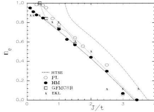
Figure 2: Several different studies results for the location of the boundary between striped and non-striped phases.  $n_e$  is the electron density,  $J/t$  is the dimensionless ratio of the spin coupling strength to that of nearest neighbor hopping. For all of these studies the boundary does exist, there is phase separation. From Carlson et al. Figure 36.
