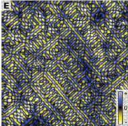
Figure 7: From [16]. Image of laplacian of tunneling anisotropy in  $\text{Ca}_{1.88}\text{Na}_{0.12}\text{CuO}_2\text{Cl}_2$  at 4.2K ( $T_c \approx 21\text{K}$ ). The color indicates the relative hole concentration. The characteristic length of structures in this image is  $4a_0 \times 4a_0$  where  $a_0$  is the Cu-O-Cu distance. According to the paper, this structure is a bond centered electronic glass. It appears to be a striped structure viewed through kaleidoscope eyes.
