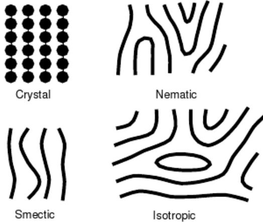
Figure 5: Cartoon illustrations of the discussed phases. Crystalline respects the discrete point symmetry of the underlying lattice. The smectic phase is translationally invariant in one direction. The nematic phase has an axis of orientation but is translationally and rotationally invariant. The isotropic phase breaks no spatially symmetries but is locally inhomogeneous. From [6]
