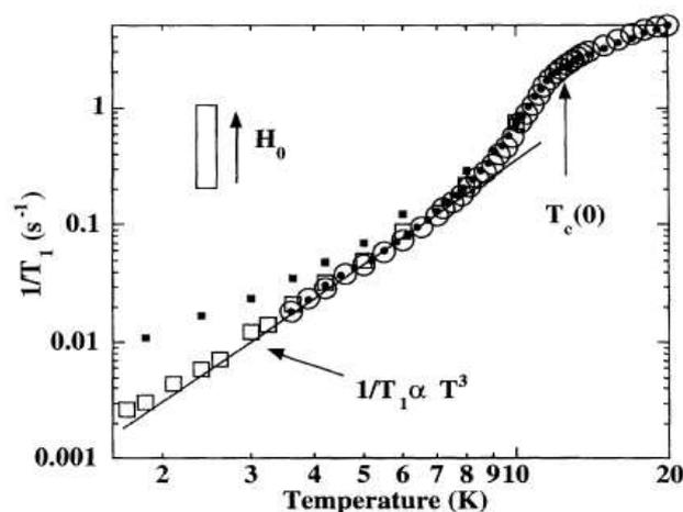
Figure 3. Data shown by Mayaffre *et al* [6].  $1/T_1 \propto T^3$  at low temperature. Spin-lattice relaxation rate decreases monotonically just below  $T_c$ , i.e. no Hebel-Slichter coherence peak.
