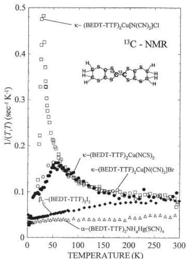
Figure 4.  $^{13}\text{C}$  nuclear spin-lattice relaxation rate divided by temperature,  $(T_1T)^{-1}$ , for  $(\text{BEDT-TTF})_2\text{X}$ . Data from Kanoda *et al.* [10].
