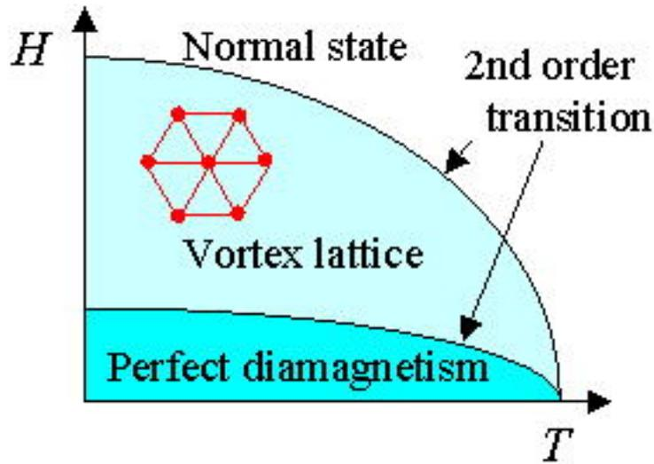
Figure 1: Phase diagram for type II superconductor
