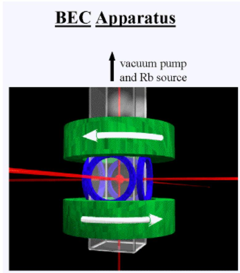
In this experiment, six laser beams intersect in a glass cell, creating a magneto-optical trap (MOT). Rb-87 atomic gases is contained in the cell which is 2.5 cm square by 12 cm long, and the beams are 1.5 cm in diameter. The coils generating the fixed quadrupole magnetic field and rotating transverse components of the TOP trap magnetic fields are shown in green and blue, respectively.
