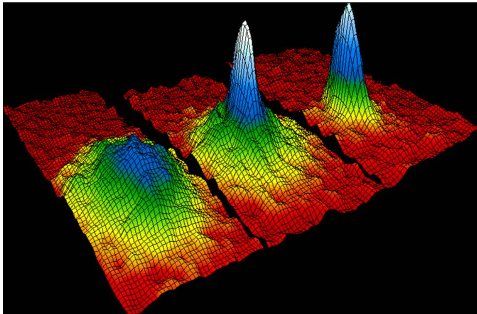
The temperature of the three plots are 400 nK, 200 nK and 50 nK (from left to right), respectively. The field of view of each image is 200 microns by 270 microns. Observation was made with laser pulse resonant with the  $5S_{1/2}, F=2$  to  $5P_{3/2}, F=3$  transition.
