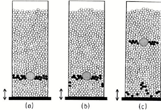
Figure 1: Convection process in a granular mixture. In (b), one can already see the fountain-like movement of the grains up the middle and down the sides; (c) shows the grains on the bottom moving towards the center and up the middle. Taken from [3].
