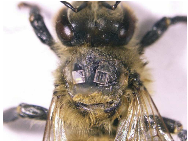
Figure 1. Typical positioning of two PharmaSeq p-chip microtransponders on the thorax of an adult worker honeybee.
