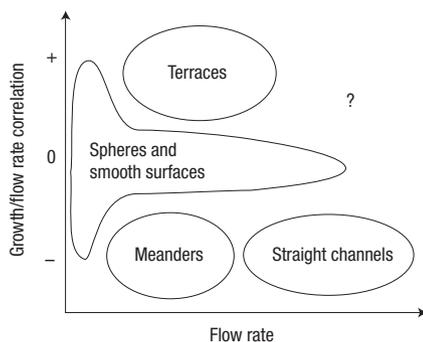
**Figure 1** Sketch of the parameter space for surface growth and erosion/dissolution under fluid flow. The upper region, where growth is faster in areas of rapid flow, is unfamiliar and little explored.
