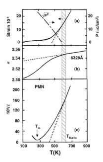
Figure 2: Deviations from linearity at  $T_d$  measured by the index of refraction and reciprocal dielectric constant [1]
