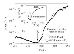
Figure 4: Temperature dependence of  $a_3$  at E = 8.5 kV/cm in PLZT at 400 Hz. The monotonic decrease of  $a_3$  is consistent with the prediction of SRBRF [7]
