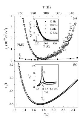
Figure 3: (a) The dielectric nonlinearities  $a_3$ ,  $\hat{a}_3$ , in PMN. Open circles are in  $E_{dc} = 0$ , open triangles  $E_{dc} = 1.5kV/cm$ . Solid squares show scanned range  $0 < E_{dc} < 3kV/cm$  for  $\hat{a}_3$ . (b) Temperature dependence of  $a_3$  based on SRBRF model, with open circles at E = 0 and open triangles at  $E = 0.85E_c$ [7]
