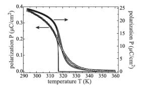
Figure 5: Polarization versus temperature or SBN:Ce of the fully poled sample (circles, right axis) and of the partially poled sample(diamonds, left axis) [5]
